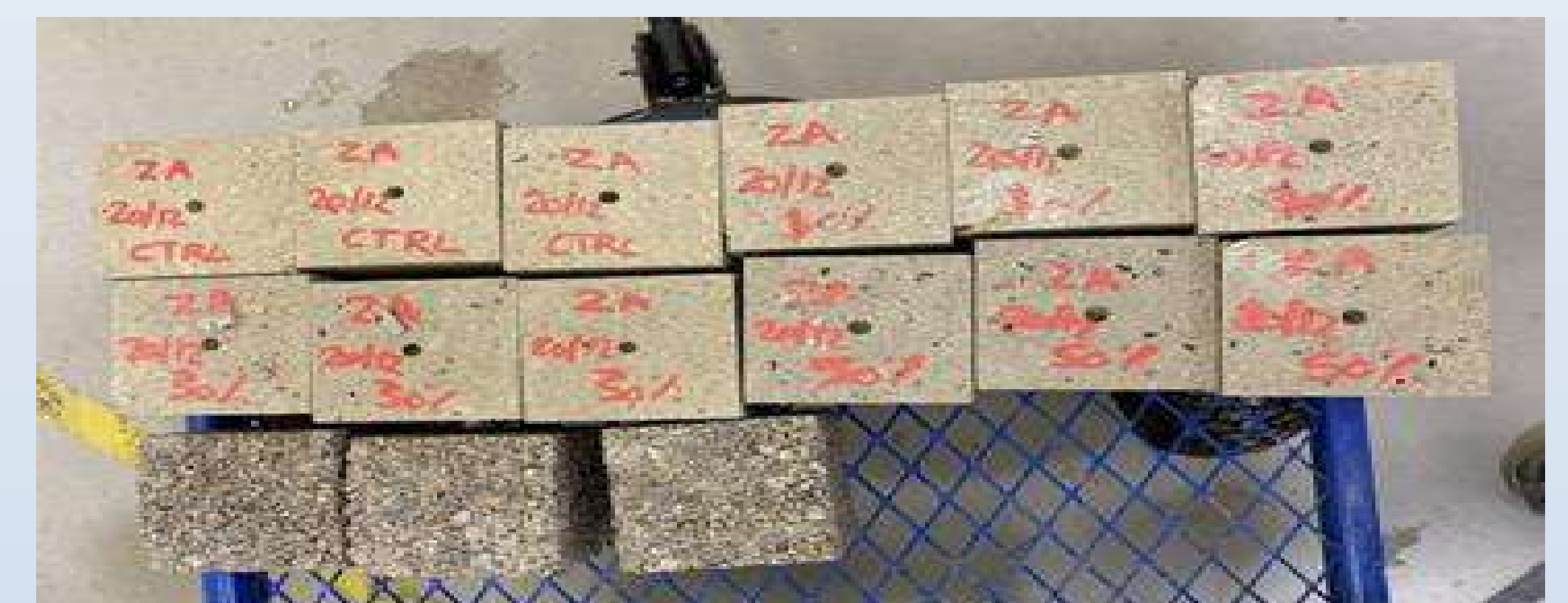
Figure 10— Concrete cubes made with various IBAA content
