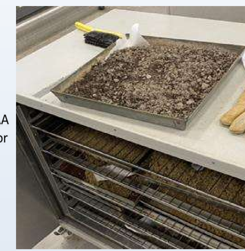
Figure 8—IBAA being dried for 24hrs
