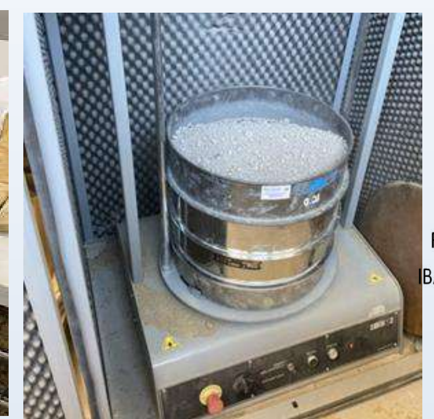
Figure 9—Sieving IBAA in different sizes once dried
