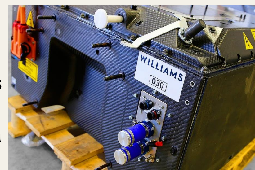
Figure 4: Formula E Battery [Source: Williams Advanced Engineering]
