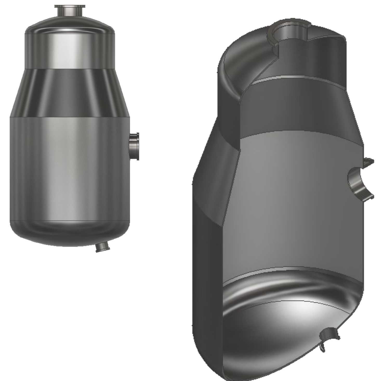
Figure 3 — Final thesis pressure vessel design created using Autodesk Inventor.
