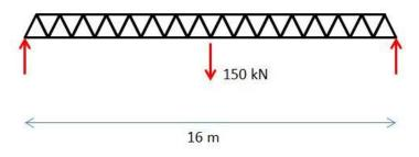
The top and bottom chords of this long truss are CHS sections, and each has  $I = 31x10^6$  mm4 and A = 6300 mm2. Take  $E_{steel} = 200$  GPa. All members have the same length of 1m. What is the approximate vertical deflection at midspan?
