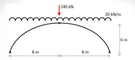
In this parabolic three-pin arch, what is the bending moment at the quarter points?
