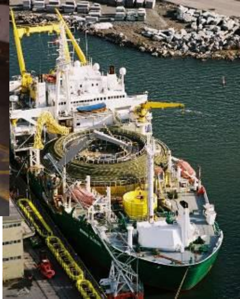
Cable carousel on Nexans Skagerrak Image courtesy Nexans
