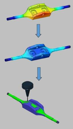
Components of the board were subjected to FEA analysis. By identifying areas of high stress under a calculated load, the design was refined to remove areas of potential failure.
