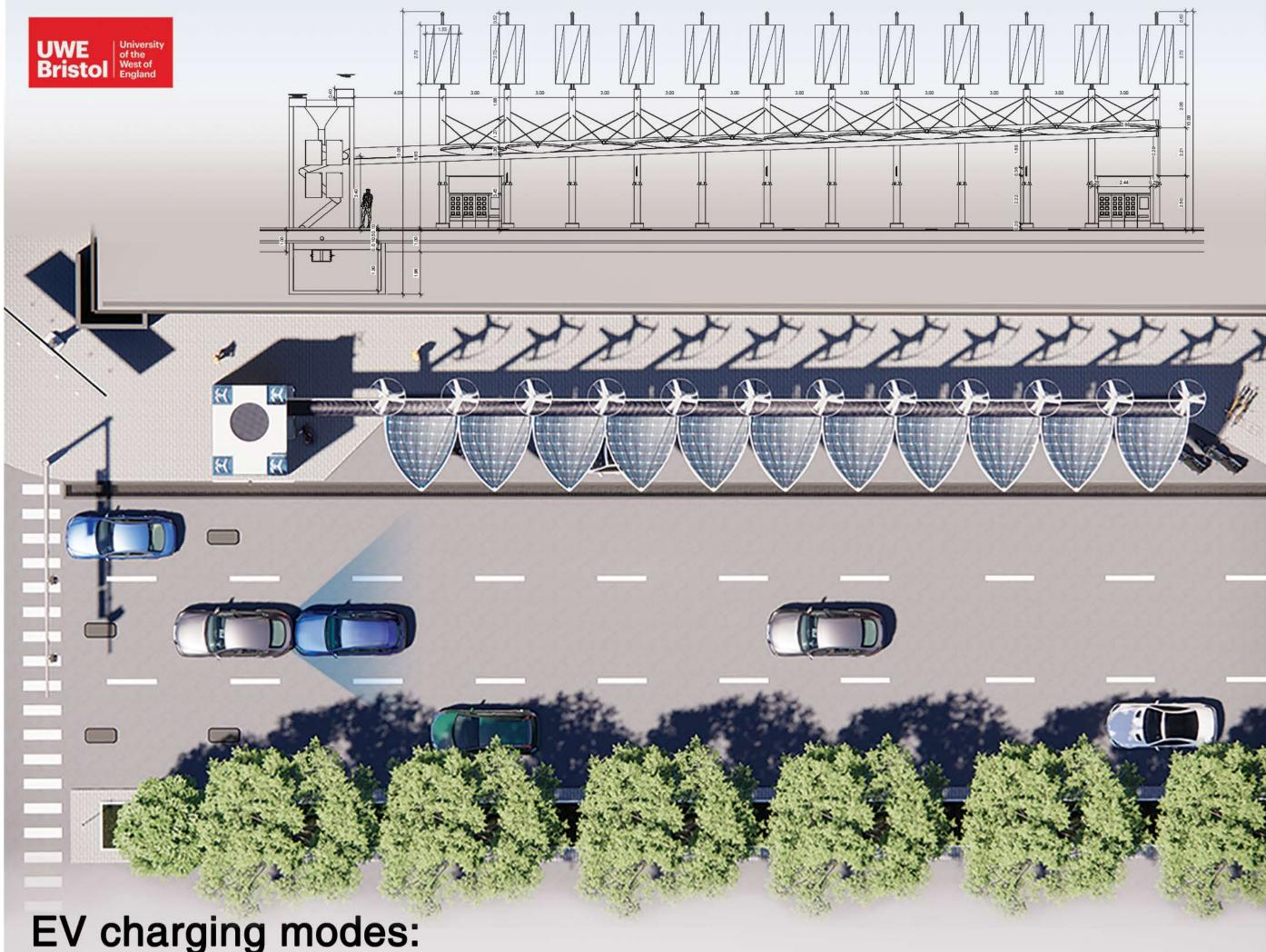
The coils are without cables, and they charge electric vehicles at the portable charging station and in the first and second rows of traffic lanes at different rates, from 3.2 to 10 kW for one coil to three coils. EVs also have car pads installed on the underside of the vehicle to receive electricity.
