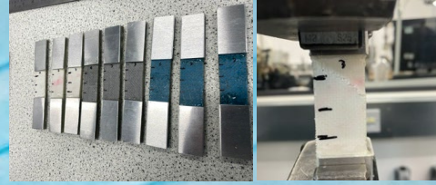
Figure 4 Tensile testing of 3 samples per each of the 3 materials
