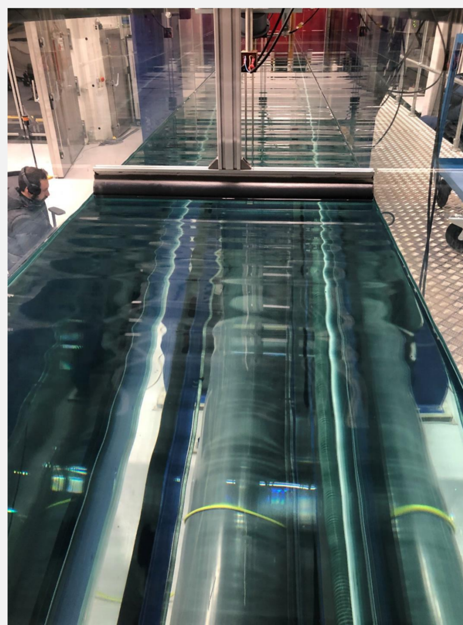
Millimetre-scale random wave generated by the wave maker
