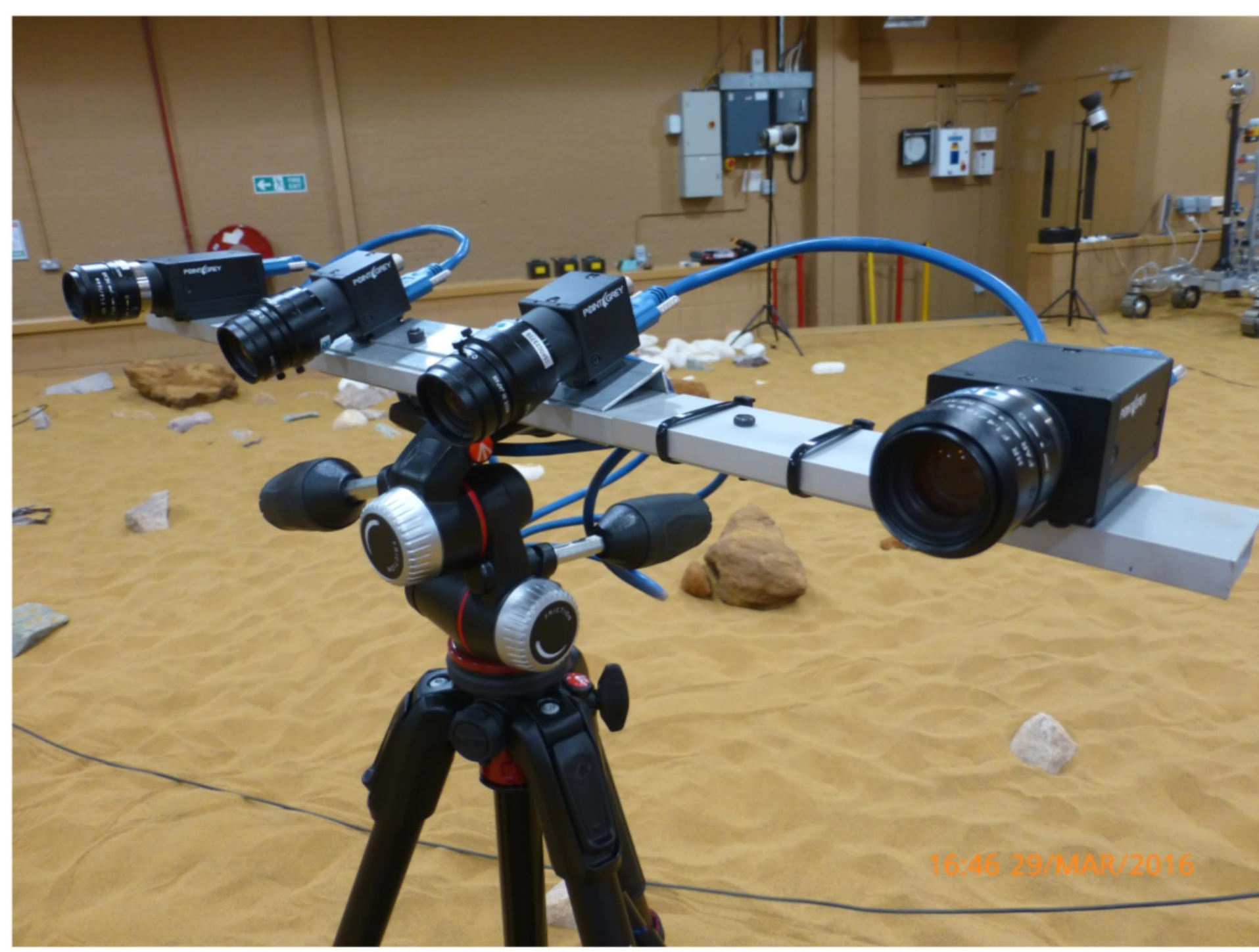
Figure 2. (left) Photo of Emulator 2. The aluminium optical bench was mounted onto a tripod, making this practical for uneven terrain such as sand.
