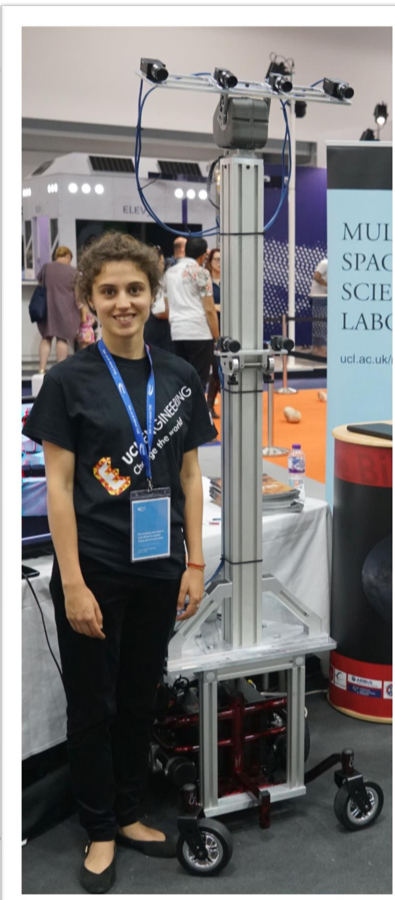
Figure 2. (left) Photo of Emulator 2. The aluminium optical bench was mounted onto a tripod, making this practical for uneven terrain such as sand.
